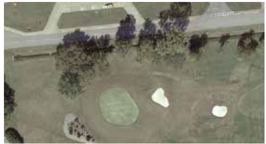
Figure 2a. Several locations of the linear hydrography feature are hidden by tree canopies. **
